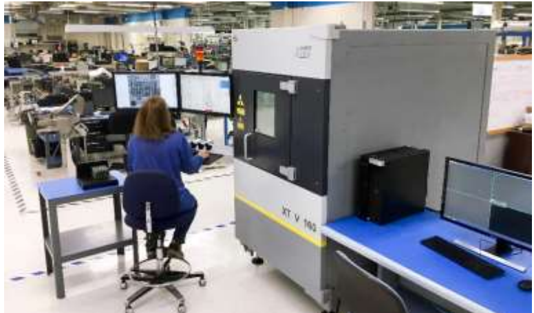
Denise Kuenzer, Senior Process Engineer, operating Lectronics' new Nikon X-ray system
