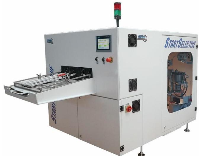
The bottom-side preheat section of the StartSelective is equipped with pulsar heaters over the full area, which can be activated individually depending on board dimensions. Pulsar heaters feature a high energy density and quick reaction time. This enables a remarkable reduction in energy consumption. An additional top-side IR preheating ensures permanent and controlled heat support during long cycles.
