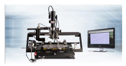
PDR's Gantry Level Focused Infrared Rework System Models E6XL and E6S are designed to rework PCBs up to 24" (610mm). PDR's unique Gantry design offers full rework access to devices placed on the leading edges of medium to large PCB formats in a simple and convenient to use rework system.
