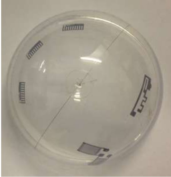
Creep Sensors, Antenna and Strain Gauge Printed on Dome with Aerosol Jet 5X System
