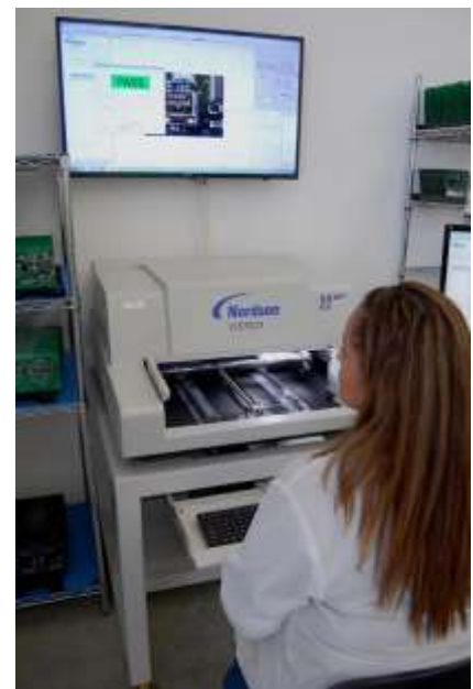
The new BX Benchtop AOI at FCI's facility
