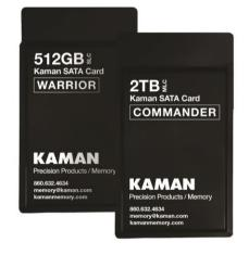
The Kaman SATA Card uses a standard ATA command set and is compatible with USB-equipped computers/laptops using a ground station adaptor. Contained in the card is an intelligent controller, including reading/writing hardware and software. The card supports declassification commands for highly sensitive applications requiring erasure of data.
