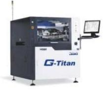
"Lights-Out-Manufacturing" with its award-winning specifications. The printer features a new interface with a modern look and many standard features, including touchscreen LCD, stencil inspection, solder paste rolling measurement, stencil lock, support block crash prevention and automatic solder paste dispense (500g jar).
