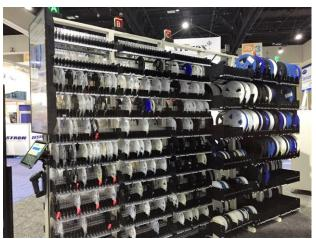
the rack by the operator. The InoAuto software tracks each individual reel, providing enhanced inventory accuracy and full traceability.
