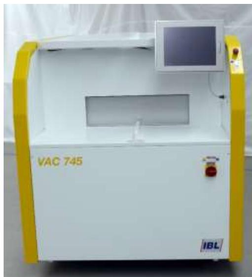
The combination of the vapor phase soldering with a vacuum process significantly increases the reliability of the finished product. Sensitive applications (e.g. fine pitch) mostly require a flexible machine with adjustable vacuum parameters. The VAC745 and VAC765 meet and exceed those requirements with the ability to influence evacuation time, holding time of the vacuum and venting time. Additionally, the patented InVapour Technology creates a fully inert soldering and vacuum process.
