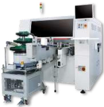
**Cypress, California – February 2018** – Hanwha’s model SM485P SMART Hybrid Mounter is designed for a wide range of applications including the processing of radial and axial through-hole components requiring controlled force insertion prior to reflow, wave or selective soldering. Innovative feeder technology features lead forming and cutting for efficient delivery of prepared components to the Mounter for quick and reliable processing.
