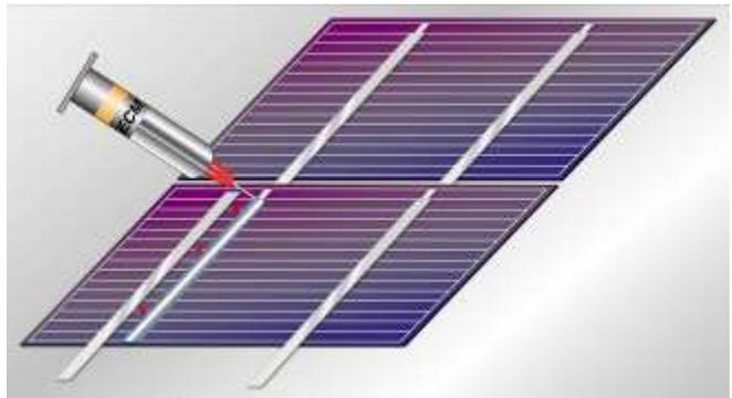
EMS materials designed for back contact applications are very flexible and cure during the encapsulant lamination process. Materials also are available with different rheologies for different dispensing techniques: Lower viscosity (screen printing or jetting), medium viscosity (needle dispensing) and high viscosity (stencil printing).
