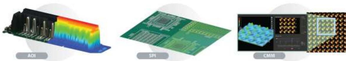
The SQ3000, deemed best in class, has been widely used for 3D Automated Optical Inspection (AOI) and can now be used for [3D Solder Paste Inspection \(SPI\)](#) for the best accuracy, repeatability and reproducibility – even on the smallest paste deposits. Combined with the award winning, easy-to-use SPI software, solder paste inspection has reached a new level of precision for the most stringent requirements.
