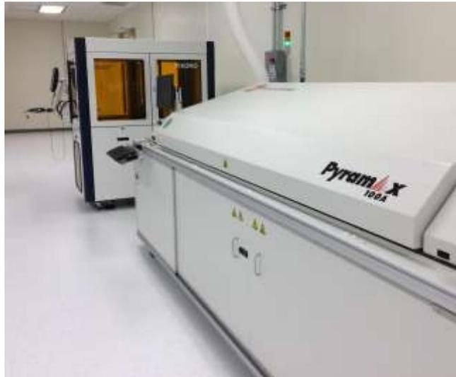
The PYRAMAX 100A was chosen for this lab because of its combination of high yield and low running costs providing a tremendous cost-of-ownership advantage. The oven features 100" of heated length and eight zones, along with 350°C maximum temperature. The system provides excellent thermal uniformity through BTU's exclusive closed-loop convection control.
