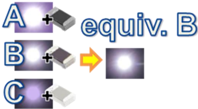
Figure 2. Correcting LED BIN by adjusting series resistance value.
