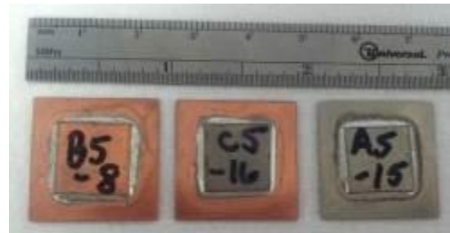
Figure 6: Samples of Void X-Ray & Electrical Test Samples
