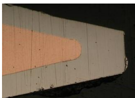
Low tip erosion after 20,000 cycles with Almit LFM-48M solder
