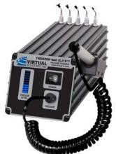
The TWEEZER-VAC Elite (TV-1500-ELITE) was developed in response to customer concerns about firmly grasping critical components and not dropping them due to a vacuum leak. This vacuum tweezer uses an integrated ten segment bar-graph display that visibly shows the vacuum level present during operation. Additionally, the vacuum port integrates a user replaceable inlet filter that protects operation of the tool from dust particles.
