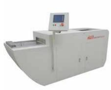
The RD2 provides consistent, uniform and reliable heat transfer for high quality reflow. With a working envelope of 18" L (455 mm) x 15" W (380 mm) x 2.5" H (63 mm), the RD2 features a patented palletized conveyor system that keeps the product horizontal throughout the process.
