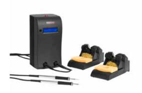
The MX-5200 features a dual-simultaneous use option, meaning that two hand-pieces can work from one power supply at the same time. The dynamic option enables the two hand-pieces to share 80 watts output power based on demand, adding even more application flexibility and speed. Four different hand-pieces and a comprehensive range of soldering and rework cartridges support the MX-5200 Series simultaneous dual operation.
