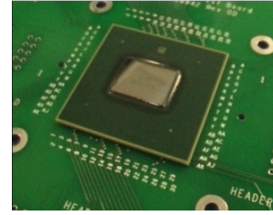
(a) Bare-die FCBGA TTV mounted to test board
