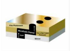
DF-3010 is the latest addition to Engineered Materials Systems' full line of film and liquid negative photo resists formulated for making microfluidic channels on MEMS devices and integrated circuits.
