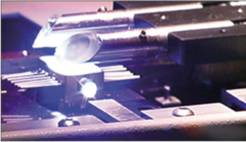
Figure 2 - In-situ epoxy cure performed by automated UV system
