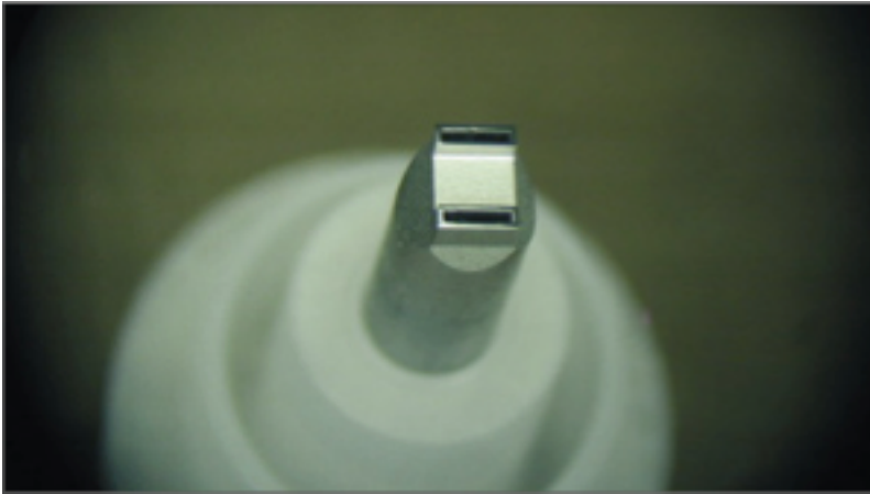
Figure 1 - Vacuum pick-up tools can be customized to pick-and-place MEMS without damaging the fragile microstructures
