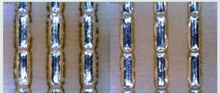
Figure 6a. Wetting pattern for SAC387. Figure 6b. Wetting pattern for Sn992.
