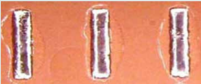
Figure 5. BiSn reflow profile and solder wetting appearance.
