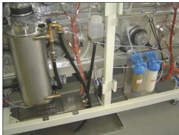
SEHO's Water Supported Process Gas Cleaning
