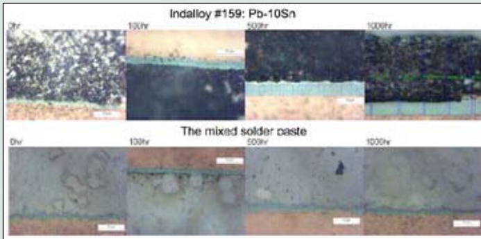
Figure 11. IMC thickness of the high lead solder and the mixed powder solder upon aging at 175oC for up to 1000 hrs.
