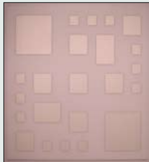
Figure 4. Customized AgPt thick film pad Al 2 O 3 substrate.
