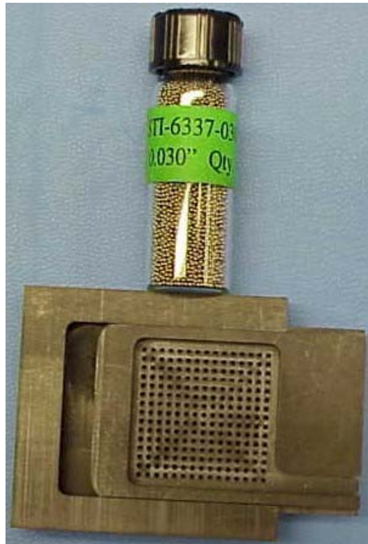
Figure 5 – re-balling fixture and solder spheres
