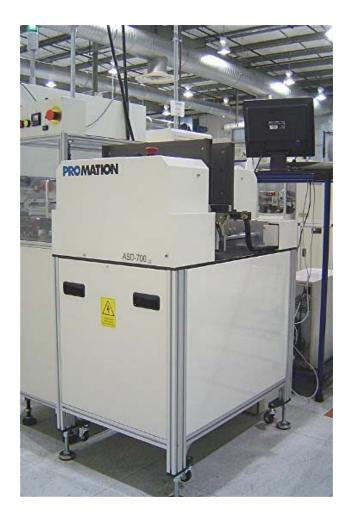
For PCBs with many holes that can not be held by vacuum, or for those customers who just prefer a mechanical de-stacking style system, The De Stacker provides a reliable means to transfer PCBs to the line.
